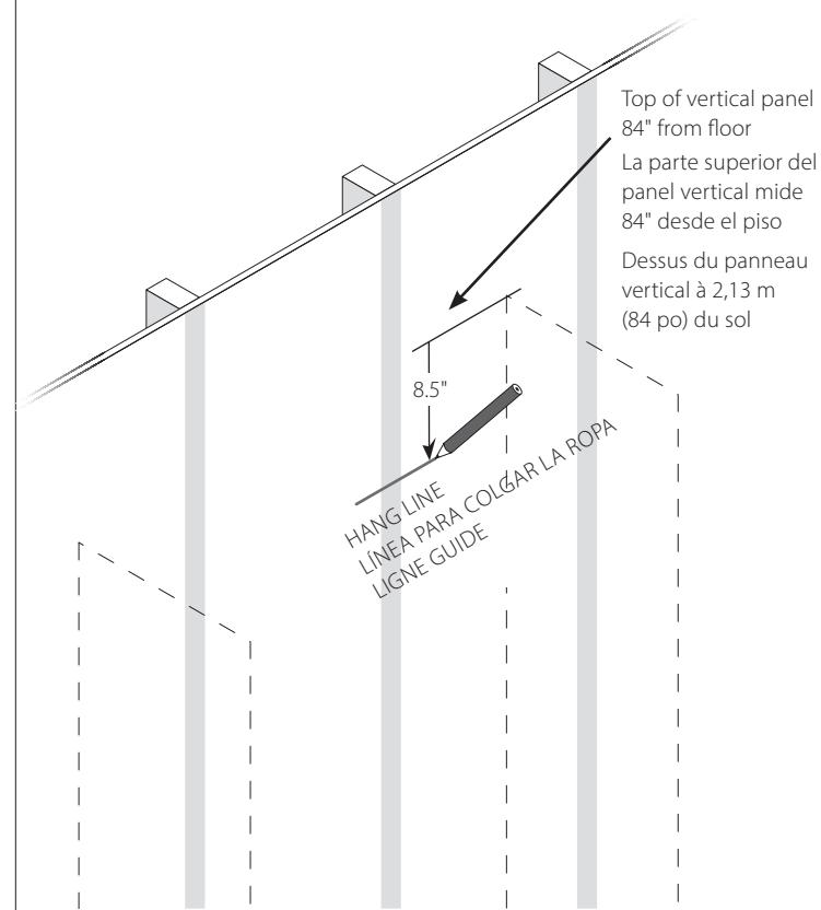
**2** Mark locations of vertical panels with masking tape.
