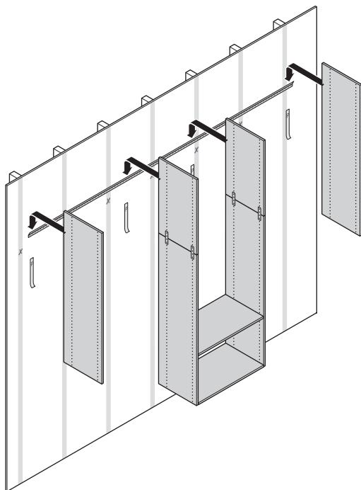
**14** Install rod holders on the vertical panels. Snap wardrobe rods into place. Install adjustable shelf with shelf pins.
