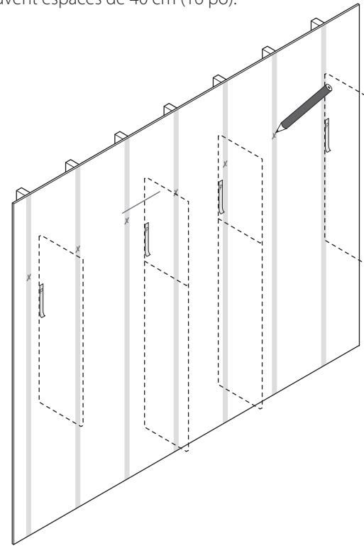
**4** Position rail slightly past outside panels. Make sure bottom of rail lines up with hang line and screw into the stud that's nearest to the center of the rail. Place vertical panel at end of rail when installing panels in a corner.
