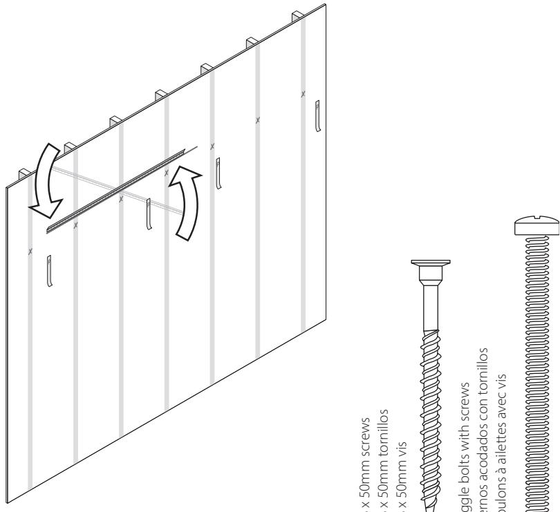
**10** Measure remaining rail and cut if necessary. Repeat steps 4–9. Cut rail to correct length with a hacksaw, if necessary.
