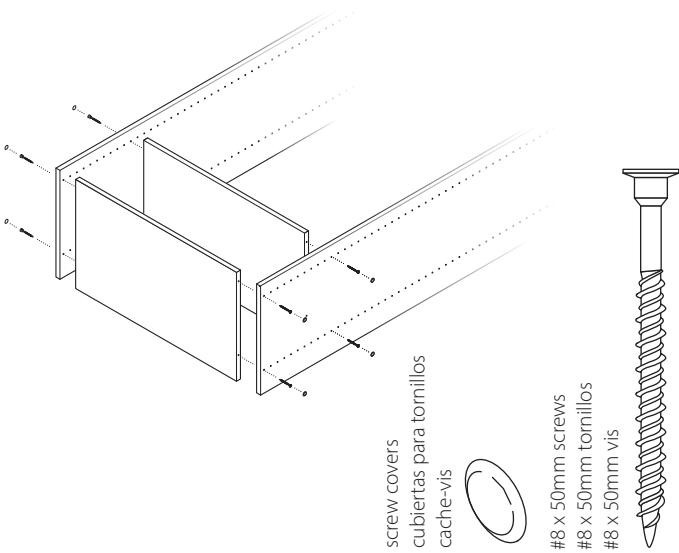
**13** Hang assembled tower unit and shorter vertical panels in their marked positions.
