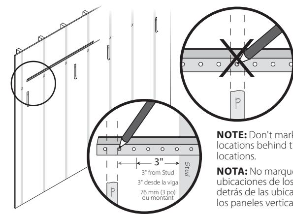
**7** Rotate rail out of position, then drill toggle holes.
