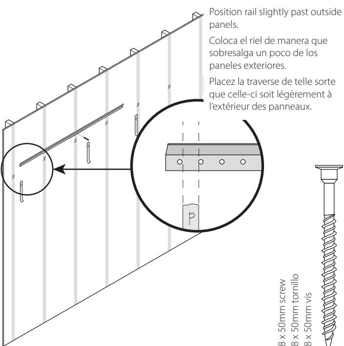
**5** Level the rail and mark a line along its bottom edge. Drill  $\frac{1}{8}$ " pilot holes into each stud location and in the last hole of the rail on both ends of the wall.
