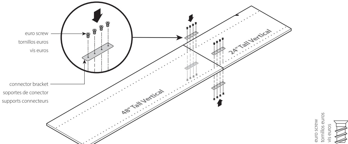
**12** To create the tower unit on the floor, attach two shelves to longer vertical panels using #8 x 50mm screws. If desired, attach screw covers onto screw heads.
