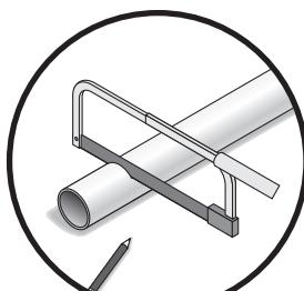
Cut rods to correct length with a hacksaw, if necessary.
