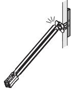
**9** Rotate rail back into position. Bolt and screw rail to wall using #8 x 50mm screw and toggle bolts if needed. Insure the rail is level when attaching it to the wall.
