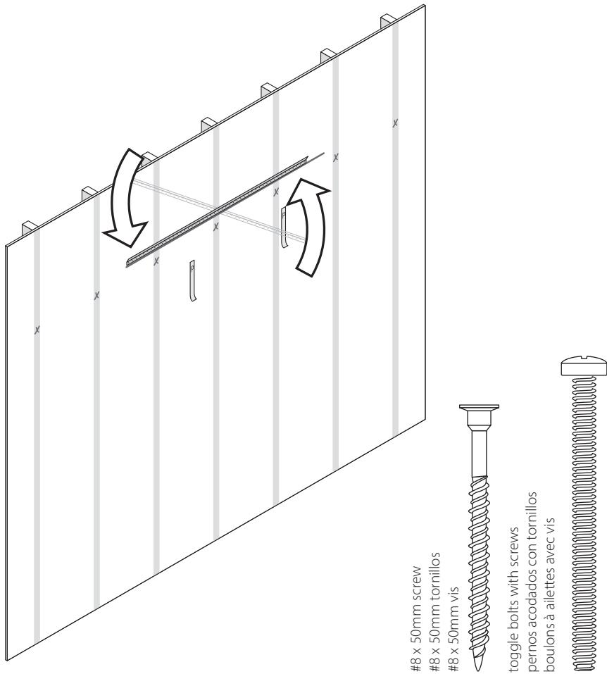
**10** Connect the 24" and 48" tall verticals with the connector brackets. Four (4) connector brackets will be used to connect each set of bottom and top verticals. Euro screws go through the bracket and into the bottom and top two (2) holes in the front and back of each vertical panel. The 24" tall vertical panels go on the top of the 48" tall vertical panels.
