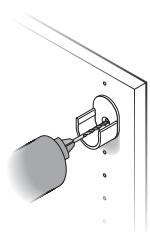
Drill  $\frac{1}{8}$ " pilot holes into vertical panels through the existing hole in rod holders.
