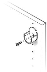
Screw rod holders to the vertical panels through the existing hole, using a #6 x  $\frac{1}{2}$ " zinc screw.
