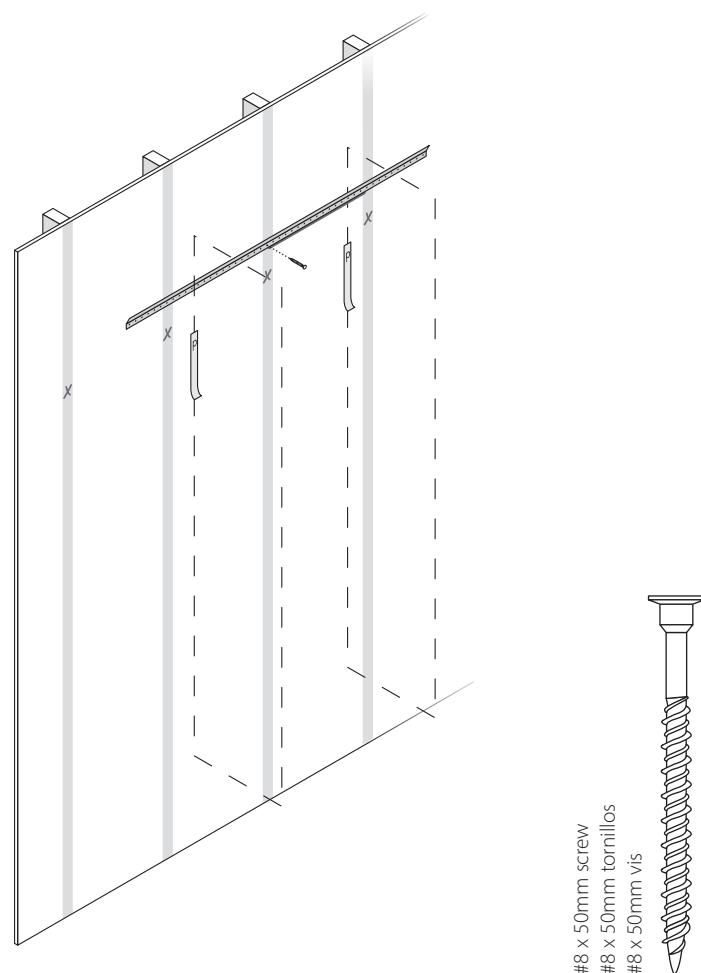
**5** Level the rail and mark a line along its bottom edge. Drill  $\frac{1}{8}$ " pilot holes into each stud location and in the last hole of the rail on both ends of the wall.
