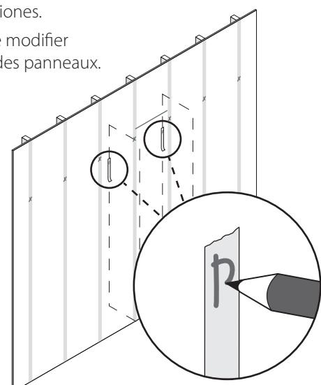
**4** Position rail slightly past outside panels. Make sure bottom of rail lines up with hang line and screw into the stud that's nearest to the center of the rail.
