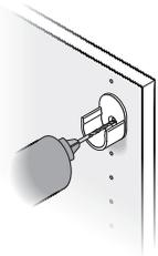
Drill  $\frac{1}{8}$ " pilot holes into vertical panels through the existing hole in rod holders.
