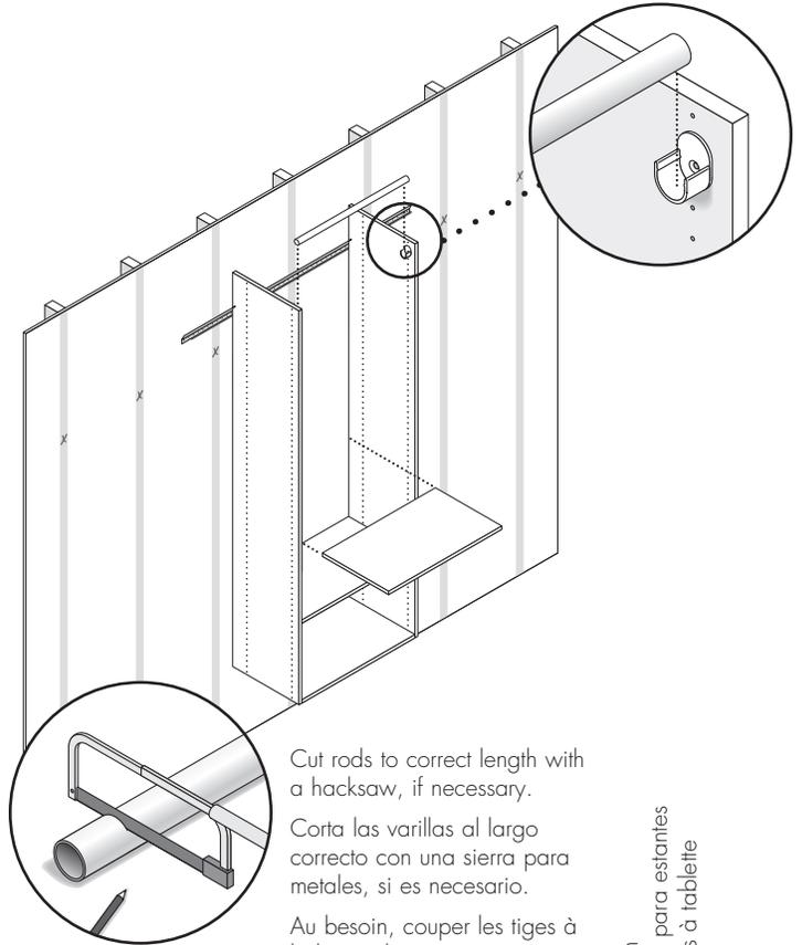
Cut rods to correct length with a hacksaw, if necessary.
