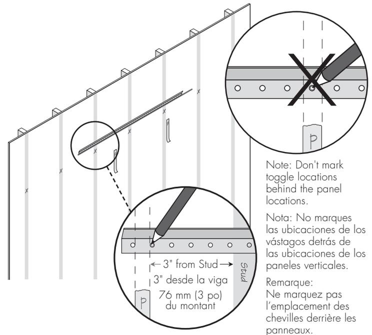
**7** Rotate rail out of position, then drill toggle holes. Use  $\frac{1}{2}$ " drill bit.
