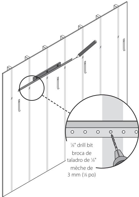
**6** **IMPORTANT.** If a vertical will be more than 3" from a stud, you'll need to use a toggle to support that panel. Mark toggle locations next to vertical panel locations. If panel will be less than 3" away, skip to Step 9.
