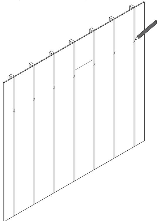
**3** Mark locations of vertical panels with masking tape.
